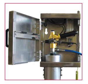
Automates the flushing process for 2K systems. Allows the use of manual spray guns with plural component spray units which automatically flush the gun when the pot life of the mixed material has expired.
